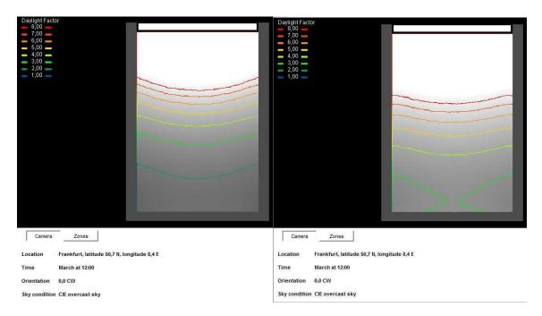
Figure 3-11 Daylight Factor calculations<sup>150</sup>, left for a cellular office with standard reflection coefficients (ceiling=0,7; wall=0,5; floor=0,2) and right for bright reflection coefficients ((ceiling=0,84(white matte); wall=0,71 (beige); floor=0,59(linoleum))
