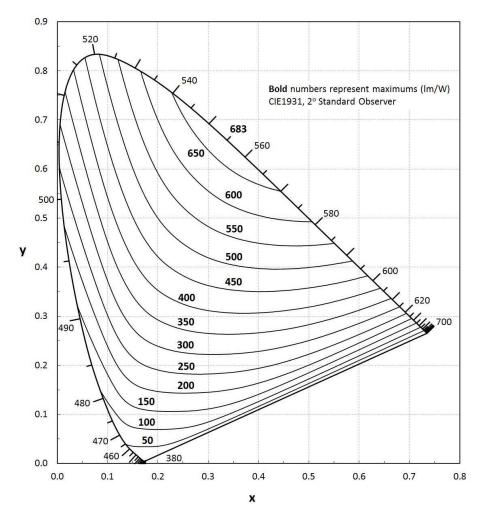
*Figure 3-17 Maximum possible luminous efficacy (lumens per watt) shown on CIE* 1931 chromaticity diagram (Schelle, 2014<sup>173</sup>)
