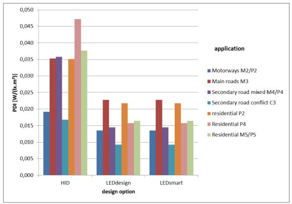
Figure 4-3 Calculated PDI values per reference road for various lighting design options
