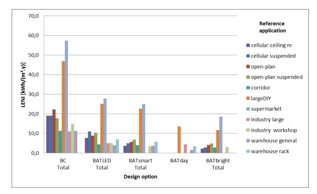
Figure 4-1 Calculated LENI values per reference indoor application for various lighting design options
