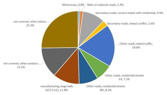
Figure 7-3 Non-Residential, Outdoor Roads and Indoor Manufacturing Halls, Electricity shares for HID-related reference cases (weighting factors for averaging of  $F_{phi}$  and  $F_{hour}$  for HID-applications).
