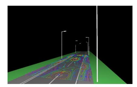
*Figure 3-15 Utilance for road lighting can be obtained from lighting design calculations*<sup>170</sup>.
