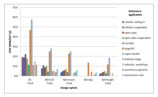
*Figure 0-1 Calculated LENI values per reference indoor application for various lighting design options*
