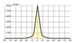
Figure 1-8: Example of a Cartesian light distribution diagram
