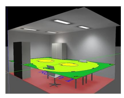
*Figure 3-13 Utilance for indoor lighting can be obtained from lighting design calculations*<sup>159</sup>.
