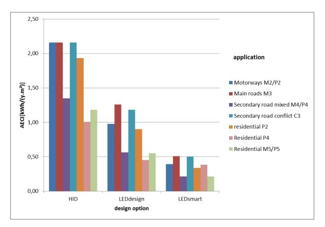
*Figure 4-5 Calculated AECI values per reference road for various lighting design options*
