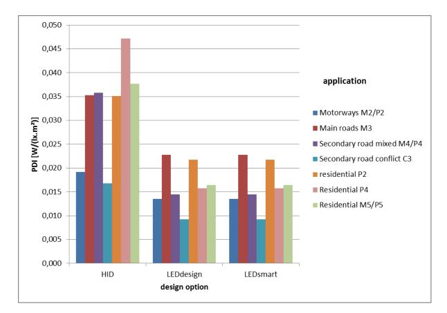
Figure 4-6 Calculated PDI values per reference road for various lighting design options
