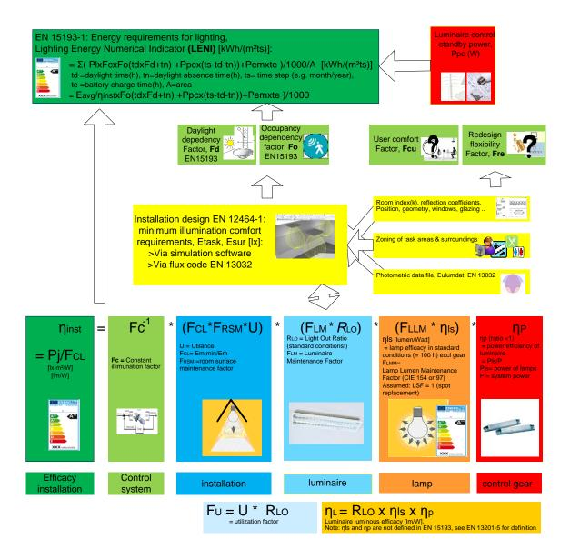
Figure 3-10 Formulas for modelling energy consumption in indoor lighting
