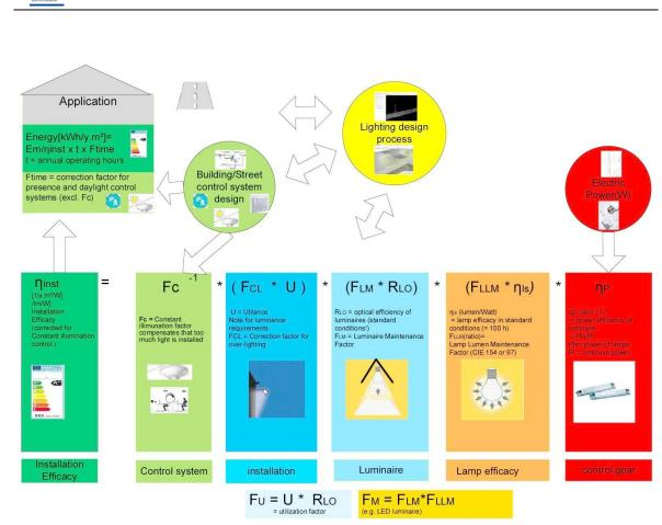
*Figure 1-1: Components of a lighting system and the most relevant performance parameters related to energy efficiency*
