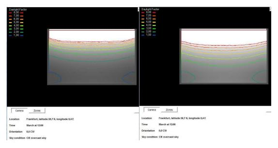
Figure 3-12 Daylight Factor calculations , left for a open plan office with standard reflection coefficients (ceiling=0,7; wall=0,5; floor=0,2) and right for bright reflection coefficients ((ceiling=0,84(white matte); wall=0,71 (beige); floor=0,59(linoleum))
